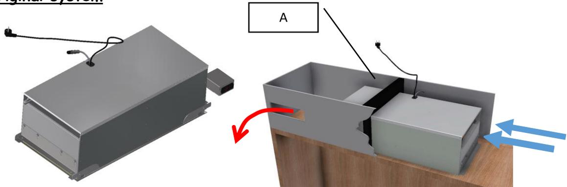
The free cross-section of each grid is 200 cm<sup>2</sup>. Separation "A" is not provided.
