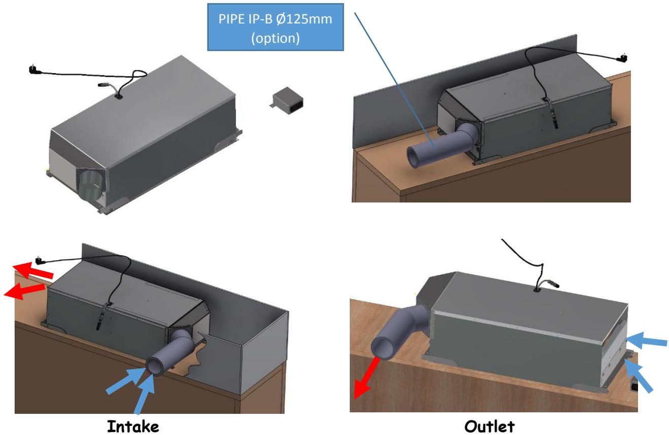
The free cross-section of each grid is 200 cm<sup>2</sup>. With the kit, the separation A is not required. **However, make sure that the distance between air intake and exhaust is sufficient to avoid that the hot air is recycle.**
